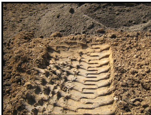
Avoid construction compaction to protect soil permeability
